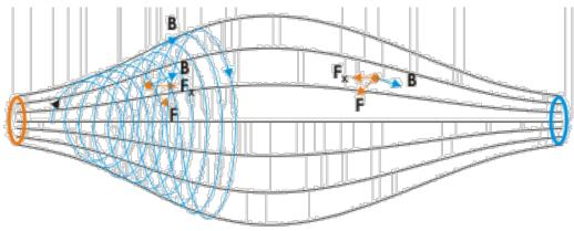
Fusion containment: the need for a magnetic bottle that reflects the charged particles.
